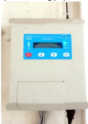
Figure 3. Web-enabled wireless remote temperature monitoring systems help continuous temperature management. However, VVMs should be controlled periodically and number of vials with VVMs reached to discard point should be reported during physical inventory and disposed of as described in the mOPV2 management guidelines.
