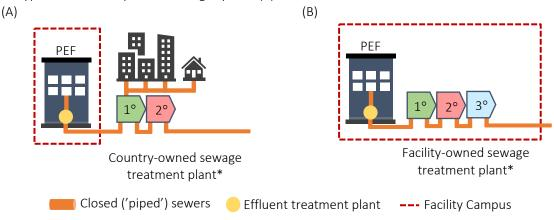
\* Sewage treatment levels: 1° (physical - settlement of suspended solids); 2° (biological - aerobic e.g., aeration tanks or anaerobic) and 3° (advanced – various types exist depending on requirements for receiving water e.g., UV, filter membranes) treatment levels. All treatment levels may include some part of the treatment process occuring in areas exposed to air e.g., aerated grit chamber, aeration tanks, aerators, etc.
